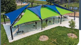
Commercial 95<sup>®</sup> is a high-quality knitted shade fabric designed for tension structures, awnings and shade covers specifically for commercial architectural applications; supplied in bulk rolls.
